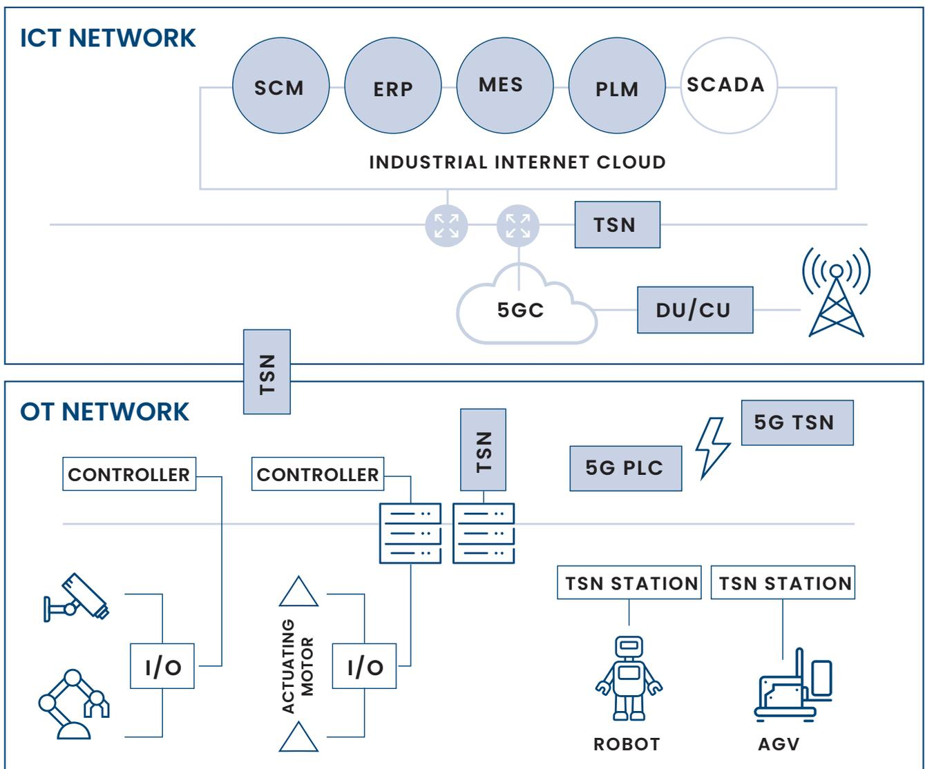
gy (IT) network and operation technology (OT) network, etc, as shown in Figure 2. 5G TSN has the characteristics of both deterministic transmission of TSN and mobility of 5G network. In the Industrial Internet, it can replace part of wired Industrial Ethernet to realise wireless and flexible manufacturing.
